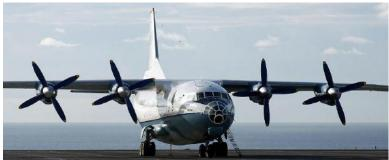
AN-12 is a specialized cargo aircraft with unmatched reliability, hot and high capabilities, and simplicity of maintenance. It has a rear ramp, spacious cargo cabin capable of carrying 20 Tons and the ability to takeoff and land from unpaved runways. 1 An-12 is currently mobilized in Africa.
