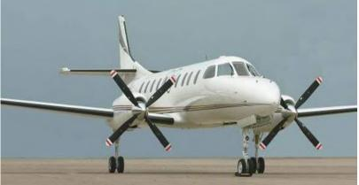
Fairchild Aerospace Metro is a 19-seat, pressurized, twin-turboprop aircraft offering a long range, low fuel burn, and pressurized cabin.
