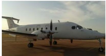
The Beachcraft 1900D is a 19 passenger turboprop with a payload of 3.5 tons capable of operating in STOL environments and all weather conditions.
