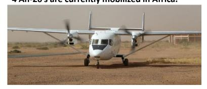
AN-28 is a high-wing monoplane with a robust tricycle non-retractable landing gear, featuring a steerable nose wheel to provide for operation from short, unprepared runways, and hot or high conditions.
