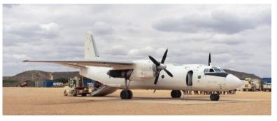
AN-26 is a medium range cargo aircraft with a rear cargo ramp for vehicles or bulk cargo. It can carry up to 40 passengers combined with cargo while operating from unpaved runways. **4** An-26's are currently mobilized in Africa.
