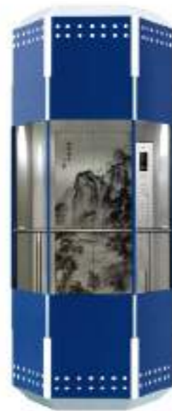
RJ108 (Optional) Car cover: Baked enamel steel, acrylic lighting decoration Observation wall: Laminated safety glass Decoration roof: Baked enamel steel frame, acrylic arch top plate with down lights Car wall: Hairline stainless steel Handrail: Stainless steel, single tube fixed on floor Floor: PVC
